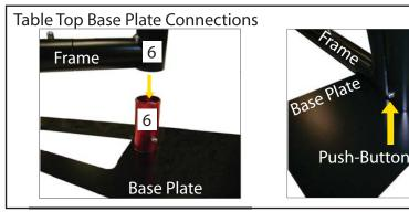
Base Plate Connections are made by holding the button down and sliding the red tube into the opposing tube on base until it locks in place.
