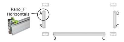
Step 2 - Place assembled vertical posts down onto corner connector on horizontal section. Do one wall or section at a time. Tighten D screws on vertical posts.
