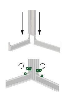
Step 3 - Top horizontal posts will have the same labels as the bottom horizontals with corner connectors attached. Slide top extrusion connectors down onto tops of vertical posts. Tighten D screws on vertical posts.
