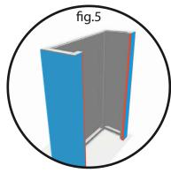
Step 5 - Insert welt in vertical grooves between top and bottom corners.
