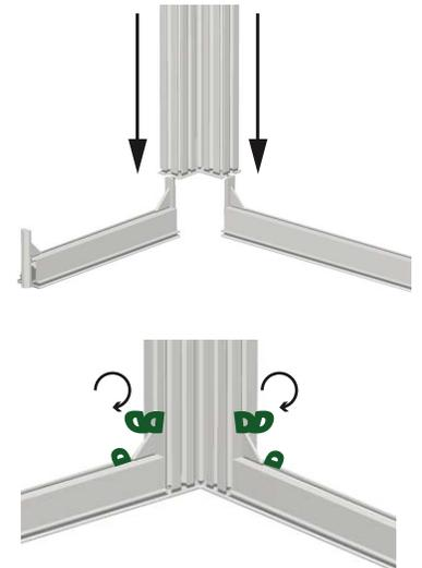
Step 3 - Top horizontal posts will have the same labels as the bottom horizontals with corner connectors attached. Slide top extrusion connectors down onto tops of vertical posts. Tighten D screws on vertical posts.
