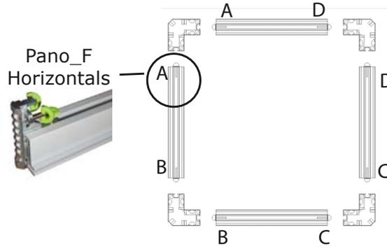
Step 2 - Place assembled vertical posts down onto corner connector on horizontal section. Do one wall or section at a time. Tighten D screws on vertical posts.
