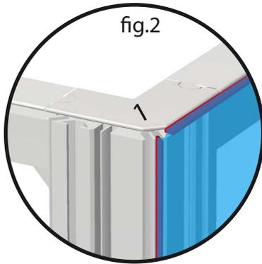
Step 2 - Insert 1 Top corner of graphic and welt into top groove of L vertical post at point 1. Align welt on left with vertical groove, insert a few inches. See fig. 2
