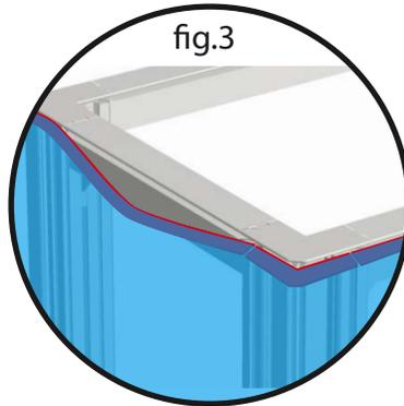
Step 3 - Align corner 2 of graphic with corner 2 on frame. Continue aligning corners around frame to final stop point.
