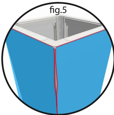
Step 5 - Insert welt in vertical grooves between top and bottom corners. Work from middle out making sure graphic is evenly distributed.
