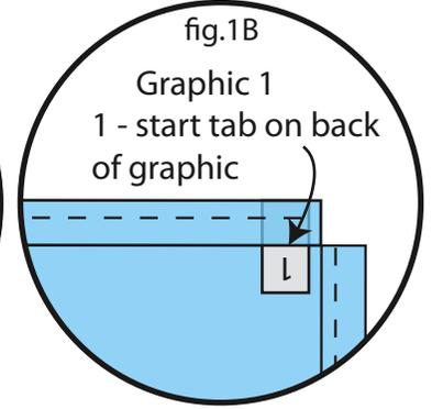
Step 1 - Identify start point on top of frame (fig. 1A, label-1) and graphic top left corner with start tab (fig. 1B, shown in blue).
